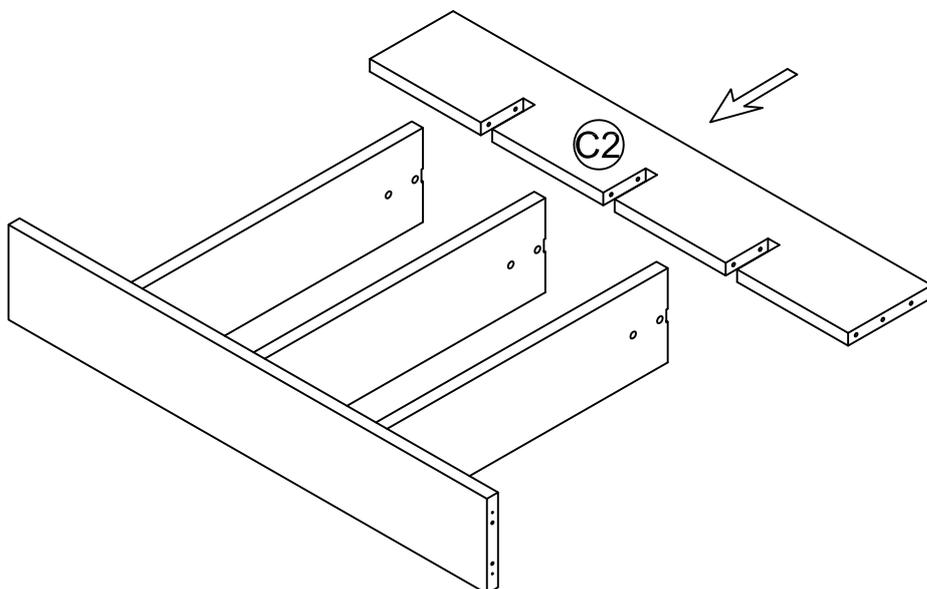
STEP 3: In the same time. Use Hex Key(G) to tighten Top panel(C3a) and Bottom panel(C3b) to Right side panel(C2) with T Nut(H) and Bolt (I). Insert Dowels(B) to Left side panel(C1), Use Hex Key(G) to tighten Top panel(C3a) and Bottom panel(C3b) to Left side panel(C1) with Bolt (E) and Washer(F)
